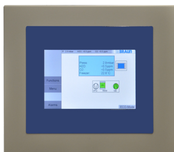
PLC - M. Braun controller with large color touch screen
