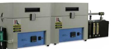
The CM190 applications and features are the same as the CM180 specifications above except it comes standard with a CM5380 Dual Zone Furnace and 5381 Furnace Kit. The CM190 system is capable of measuring organic and non-organic surface carbon.
