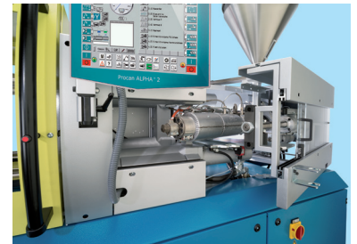
The swivel-out injection unit facilitates alterations and maintenance
