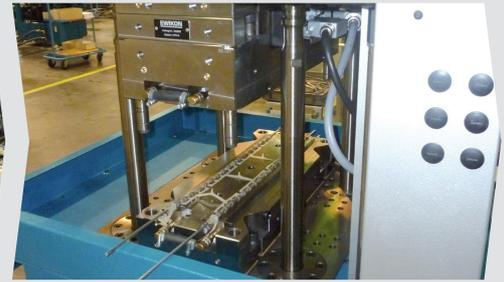
Continuous production of distance pieces of saw chains
