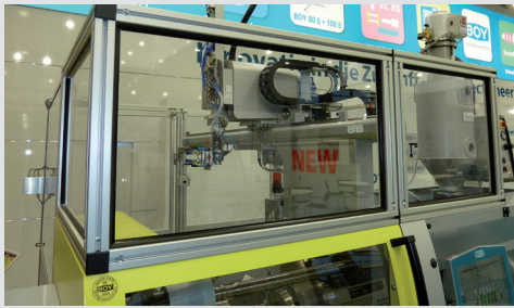
Four-axis industrial robot integrated on top of the clamping unit.
