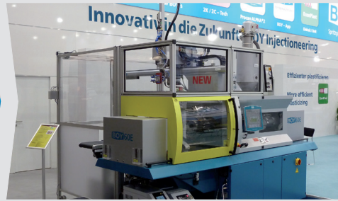
Production cell with CE-compliant safety housing
