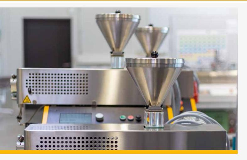
Collin Teach Line is a series of compact table-top machines for the processing of polymers especially for apprenticeship & training as well as research & development.
