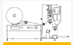
At low-viscose melt, for casting to the lower cooling roll, the die is arranged e. g. at an angle of 90°.
