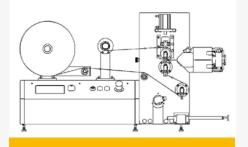
For smoothing, the upper roll is deepened pneumatically to an exactly adjustable roll gap. An unwinding station, which is arranged above the die, allows to laminate sheets with polymers.
