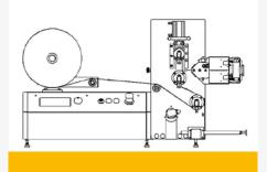
At the upper roll swiveled up, with the horizontally arranged die, the film is pulled via the center roll. Here, the center roll is tempered, the lower roll is cooled.
