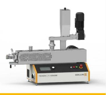
All Collin compounders are available for co-rotating or counter-rotating operation and can be retrofitted. The table-top compounder consists of a processing section with drive, mounted on the electric control cabinet.
