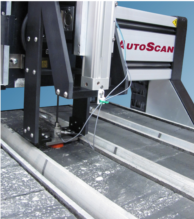
The impulse hammer probe is used to characterize the variability of elastic stiffness and mechanical strength
