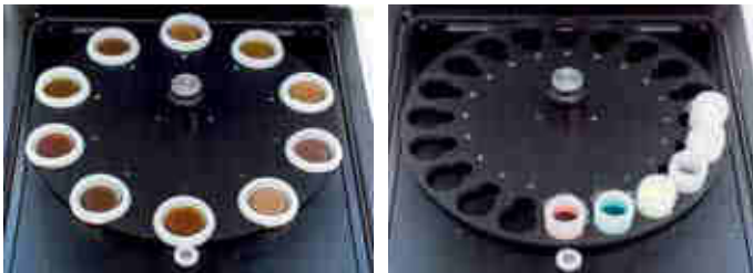
10-position and 20-position sample changers.
