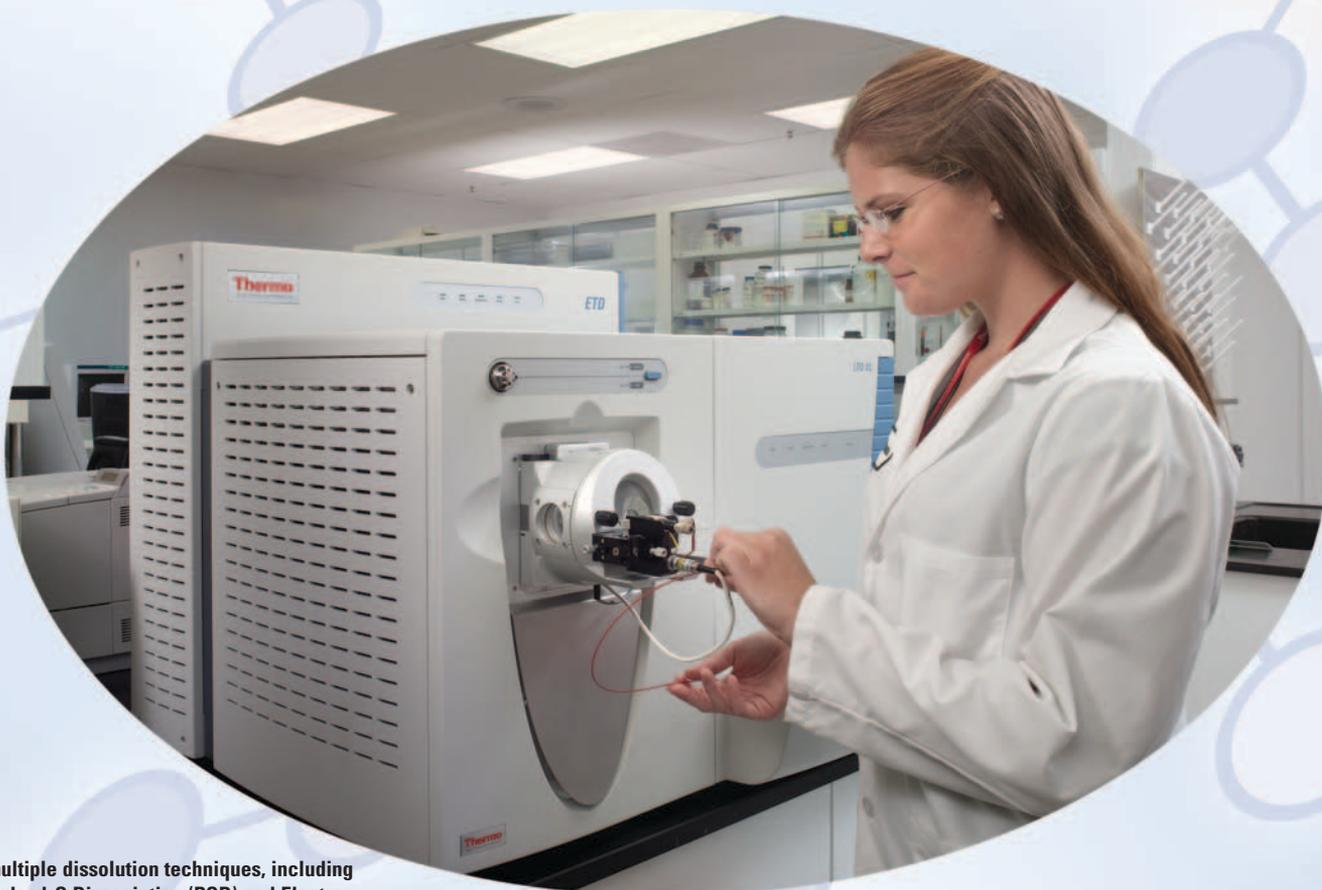
Using multiple dissolution techniques, including Pulsed-Q Dissociation (PQD) and Electron Transfer Dissociation (ETD), the LTQ XL generates extensive structural information for the most demanding proteomics samples.
