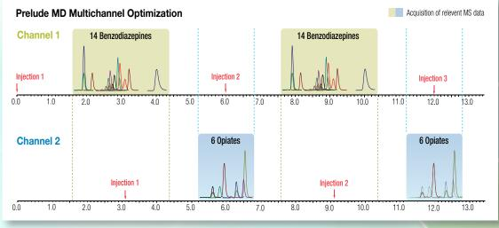
Multichannel optimization allows you to maximize mass spectrometer use and throughput.
