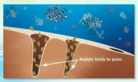
Large compounds flow to waste. Small compounds diffuse into pores. Only those small molecules that have an affinity to the chemistry inside the pores bind to internal surface. Other small molecules with a lower binding affinity quickly diffuse out of pores and are flushed to waste.
