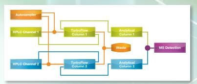
The autosampler injects samples into the TurboFlow columns for cleanup. Then the HPLC pump delivers the analytes of interest to the analytical columns for separation. After separation, analytes are delivered to the MS for detection.
