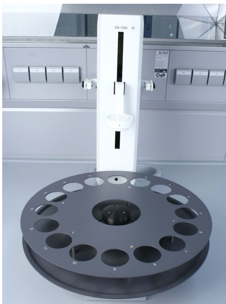
Fig.1: TW 7200 with 16 position sample tray and titration head TZ 1463
