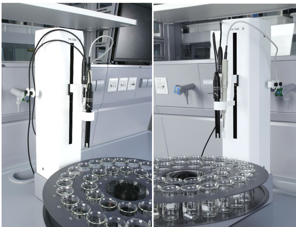
Fig. 5 a/5 b: TW 7200 with 38 sample tray TZ 4038, titration head TZ 1469 (new version) pH-Micro - and conductivity electrode SCPpHT-MIC-AMF-3M-DIN-N and LF 413T-3M ForkIDS.
