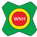
Non-Potable Water, Hot
