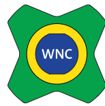
Non-Potable Water, Cold
