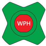
Potable Water, Hot
