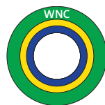
Non-Potable Water, Cold
