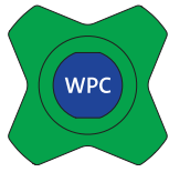
Potable Water, Cold
