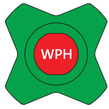
Potable Water, Hot
