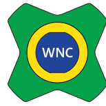
Non-Potable Water, Cold
