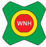
Non-Potable Water, Hot
