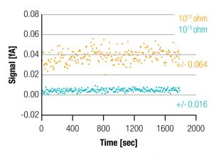
Heavily reduced signal to noise with  $10^{13}\,\mathrm{ohm}$  amplifier
