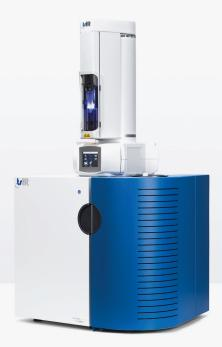
The TSHR Total Nitrogen Analyzer, model TN 7000, is able to detect fast and accurate trace level nitrogen concentrations in a wide range of liquids and LPG/Gas sample types. The analyzer is designed to facilitate the current and future demand of total nitrogen analysis down to ppb level.
