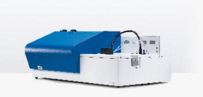
The sample is introduced by a fully integrated automatic boat/syringe driver, into a heated oxygen free environment to ensure a complete vaporization of the sample. The carrier gas ensures that the vaporized sample will transfer into the combustion zone where oxygen will be added to complete the oxidation of the sample. After the dual zone combustion stage, the combustion gasses flow through a perma-pure dryer tube where all moisture and other potential interferences are removed.
